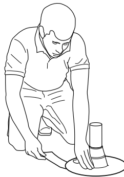
Slowly pull the release paper to expose the seam tape
