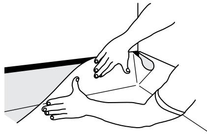
Press the second side against wall, forming an “ear” at the corner.
