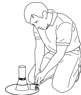
Roll firmly with a steel roller to bond the boot to the roof sheet.
