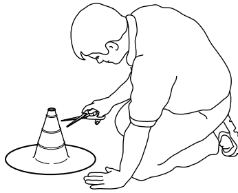
Cut just above the molded ridge corresponding to the desired pipe size
