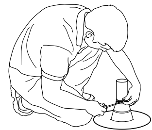
Screw the hose clamp around the top of the pipe boot.
