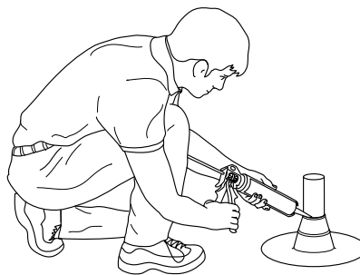
After cleaning the top of the boot, caulk between the boot and pipe.
