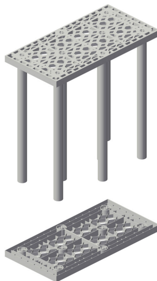
STEP 2: Flip the assembly and insert the support columns into the sockets of the second top/bottom plate.
